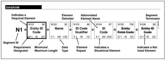
Figure 2.4. Segment Key — Diagram
